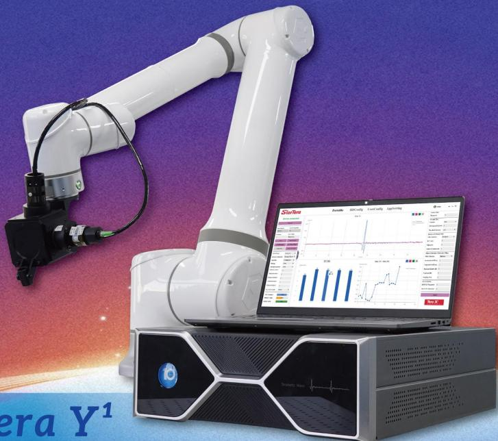
A robotic arm carrying a THz sensing head enables precise, repeatable, and flexible scanning of complex targets. Combined with **AI** algorithms, the system can automatically identify hidden defects, material changes, and early-stage anomalies from THz data.
